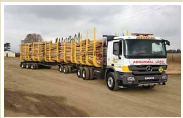
67 ton PBS Timber Vehicle operated by Zabalaza Transporters which has been introduced in KwaZulu-Natal as part of the Performance Based Standard Pilot Project
